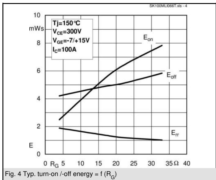
Fig. 4 Typ. turn-on /-off energy = f ( $R_G$ )
