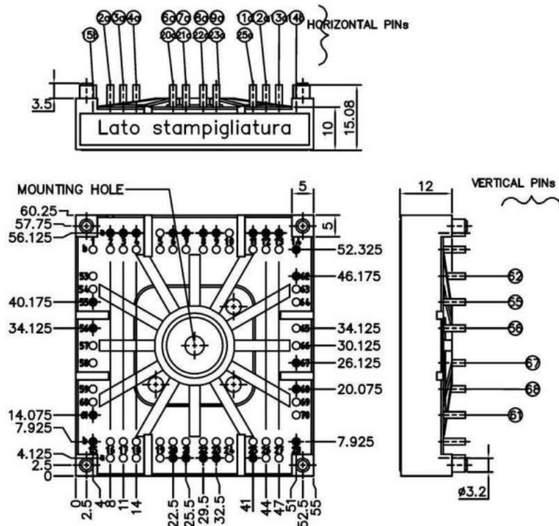
Case T 88 (Suggested hole diameter for the solder pins in the circuit board: 2mm. Suggested hole diameter for the mounting pins in the circuit board: 3,6mm )
