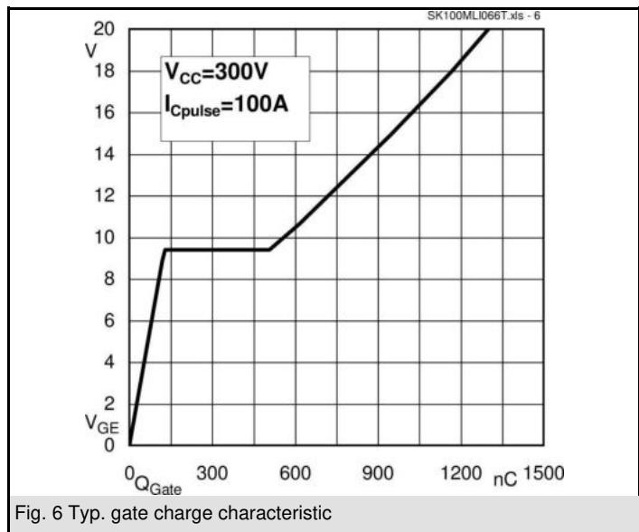
Fig. 6 Typ. gate charge characteristic
