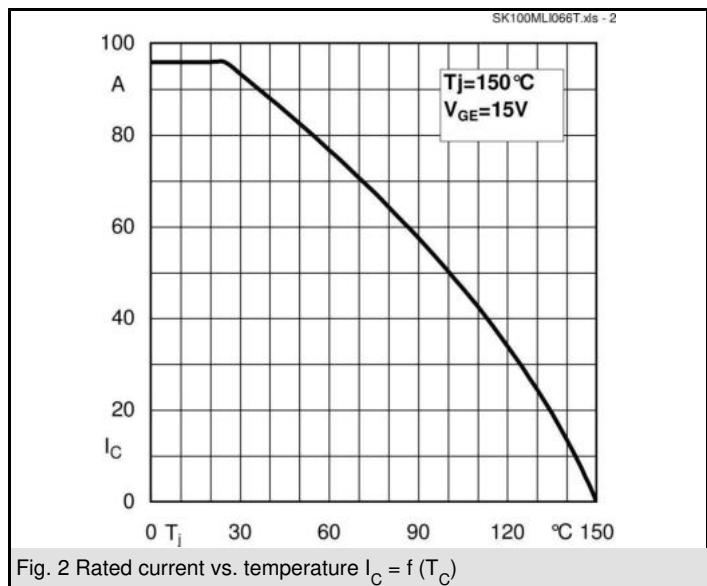
Fig. 2 Rated current vs. temperature  $I_C = f (T_C)$
